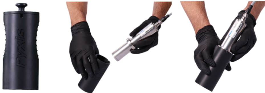
Figure 18. LT-73X Series sensor use with T-CAL kit
